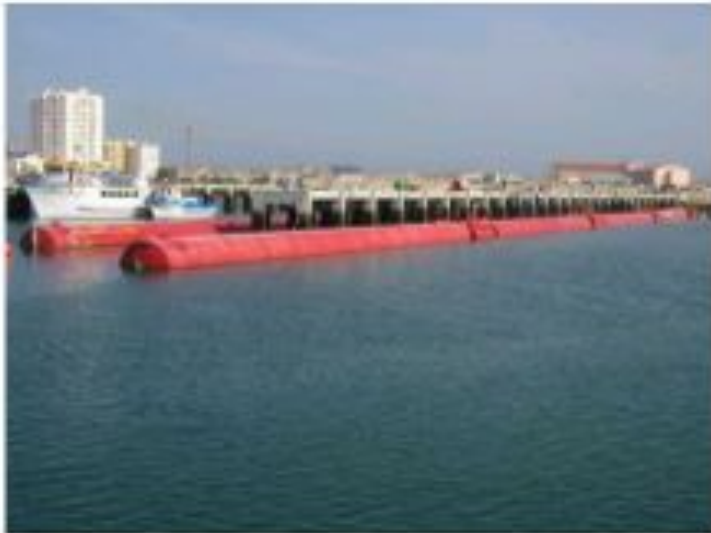
Pelamis Wave Energy Converter P 750, Orkney, Škotska, 2007, 750 kW
